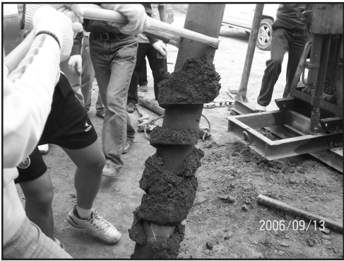
图 3 现场试验中粘在螺旋叶上的土被取掉 Fig 3 Drilling Test of Dual Tube Auger: the Soil Cohered on the Flight of the Outer Wall was Taken Off
