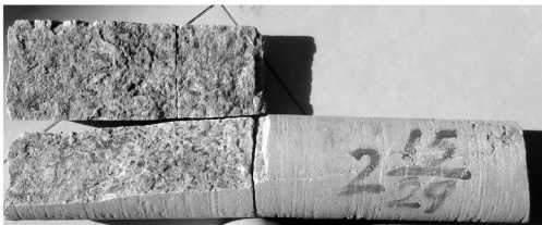
图 2 桦 3 井长 2 22 油层砂岩中的张性裂缝 Fig. 2 Tensional Fractures in the Chang 2 22 Oil bearing Sandstone of Hua 3 Well
