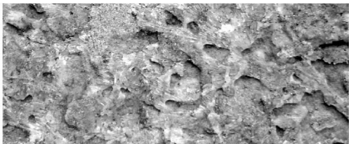
图 3 桦 3 井长 2 22 油层砂岩张性裂缝充填物表面放大 Fig. 3 Enlarged Surface Image of Fillings in Tensional Fractures in the Chang 2 22 Oil-bearing Sandstone of Hua 3 Well
